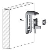
Recommended fixing countersunk screw type - head Ø 5 mm max.
